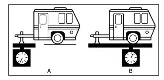
The trailer tongue weight (A) should be 10 percent to 15 percent of the total loaded trailer weight (B), up to a maximum of 600 lbs (272 kg) with a weight carrying hitch. The trailer tongue weight (A) should be 10 percent to 15 percent of the total loaded trailer weight (B), up to a maximum of 1,000 lbs (454 kg) for the 1500 series and up to a maximum of 1,500 lbs (680 kg) for the 2500 series with a weight distributing hitch.
